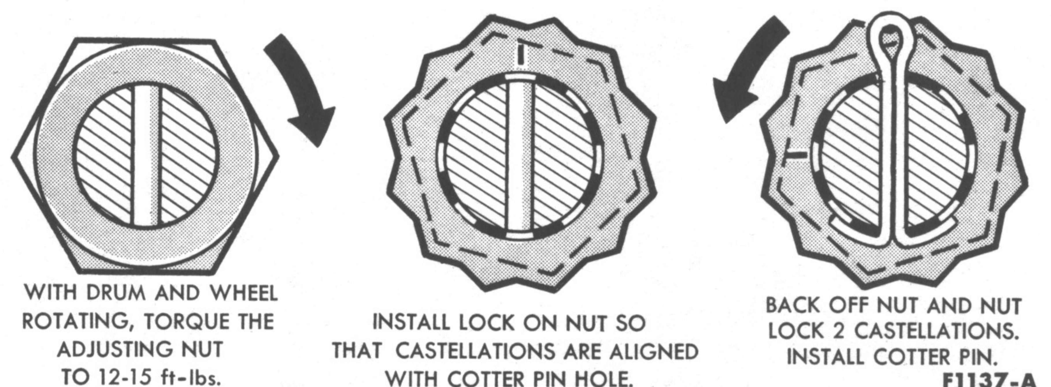
FIG. 58—Front Wheel Bearing Adjustment
